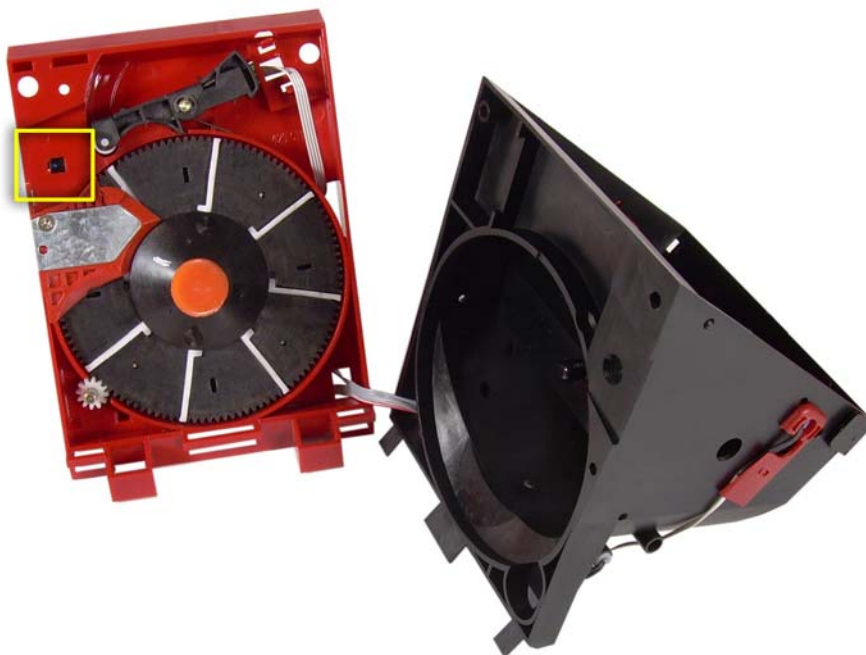
Figure 27. Cleaning of the Hopper U-II
