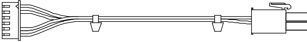
P/N 09280034 SIGMA GAMES INTERFACE FOR IC-16 TO REPLACE CC-16, 12VDC, INHIBIT HI, SENSE (SR)
