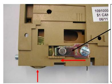
Insert a \$1 Canadian coin up through the reject path slot as shown.
