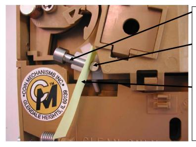
Adjust magnet by sliding it in the white plastic holder so that there is a small gap between it and the
