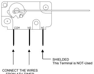
FROM ATV-TIMER TO THE COIN MIRCO-SWITCH "COM" AND "NO" TERMINALS
