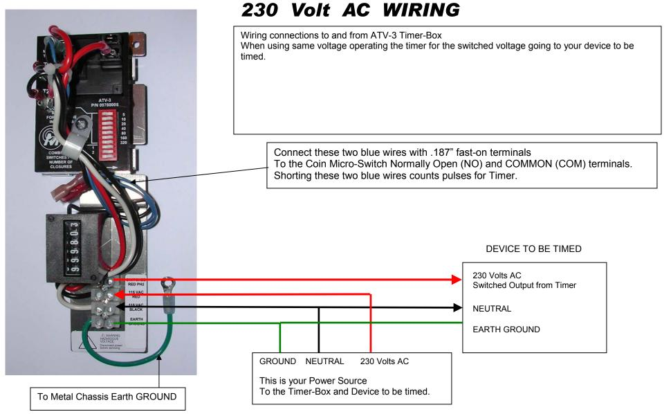
Ground wire is earth ground and is shown for safety.
