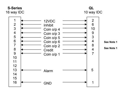
**Note 1** : When using the harness to replace an S-series validator, ensure that the QL output line 4 is connected to the S-Series Pin 6 (coin output 6) or Pin 8 (accumulator/credit) depending upon the application.
