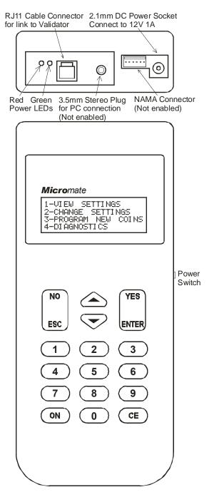
The Micromate 2.0 is connected to a QL validator via the supplied RJ11 cable. A VAL365 interface is used to further interface with a QL3 JST connection. It is recommended that the validator is powered from a 12Vdc 1A power supply via the parallel port. This will supply power to the validator, and also power the Micromate via the RJ11 comms cable. The validator may need to be enabled by connecting the INHIBIT (pin 6 on a 10 way header) to 0V (pin 1 on the 10 way).
