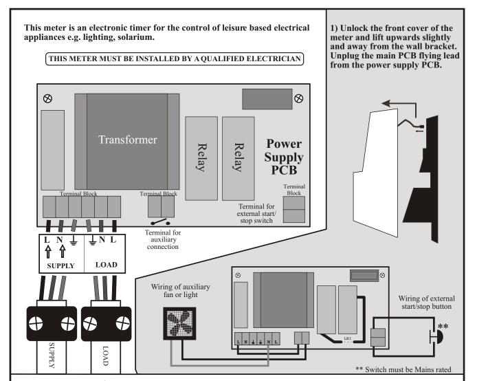
\* If the meter is an 030/4/7102 or an LT3100/LCB (Large Coin Box) Please use these instructions together with 030/1/9008 installation sheet.
