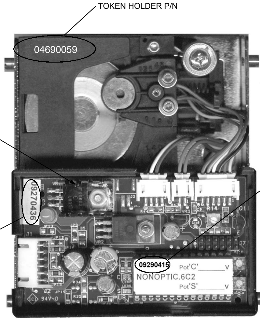
IC-37 WITH COVER REMOVED
